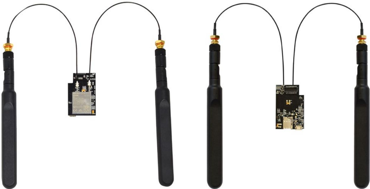
Figure: NB-IoT / Cat-M module antennas
